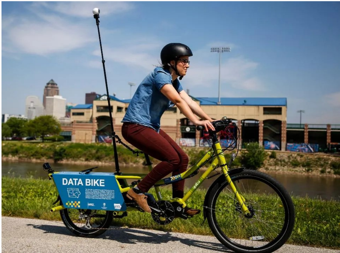
Trail mapping will begin in the summer of 2025. R1's bike will be modeled after this one, built and used by the Des Moines Area MPO. The electric bike features a 360-degree camera to record images for Google Street View, an iPhone to record pavement roughness, and a rear-facing GoPro camera to photograph trail conditions. Photo from the Des Moines Register, May 19, 2017
