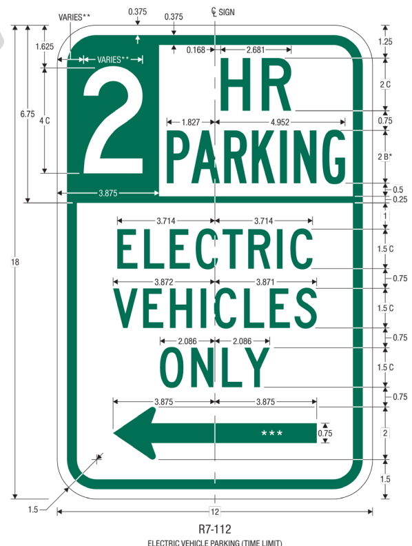
On-Street Electric Vehicle Charging (R7-112) plaque, Manual of Uniform Traffic Control Devices for Streets and Highways. Source: FHWA
