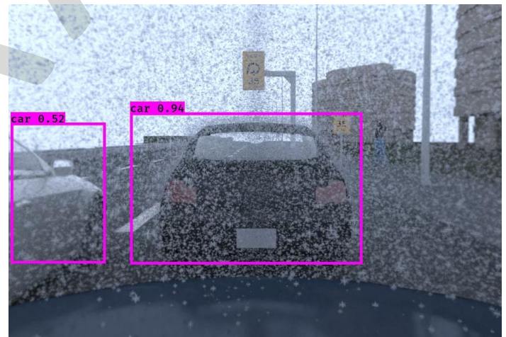
Image 2-8: Obstructed CAV Sensor
